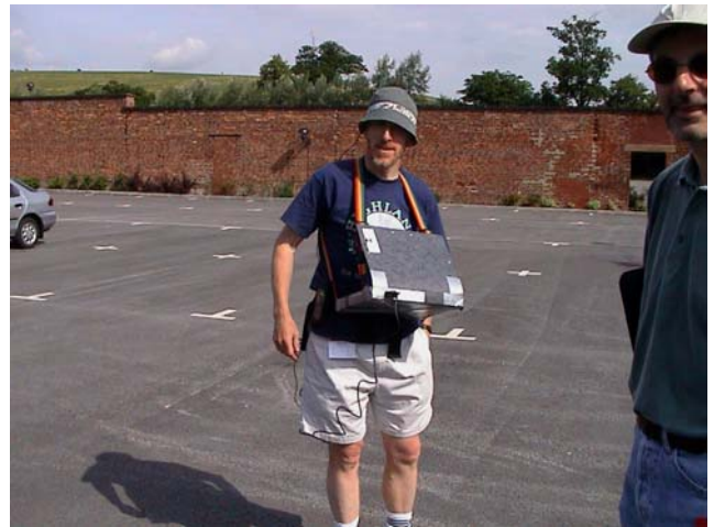
Figure 10 – Field Equipment – Laptop, Receiver and Antenna (under Hat).
