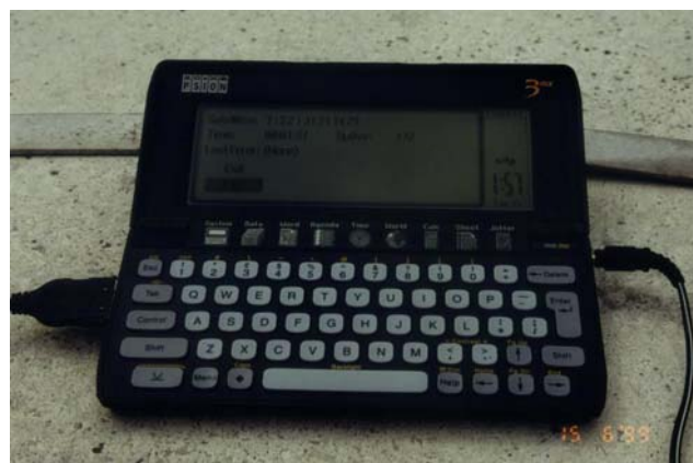
Figure 5 - Logging Data to a Psion PDA
